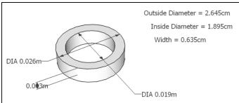
Figure drawn with Google Sketchup, Sketch dimensions in meters. Use the more exact dimensions listed in upper right this will be easier since density is in cubic cm or  $cm^3$ .
