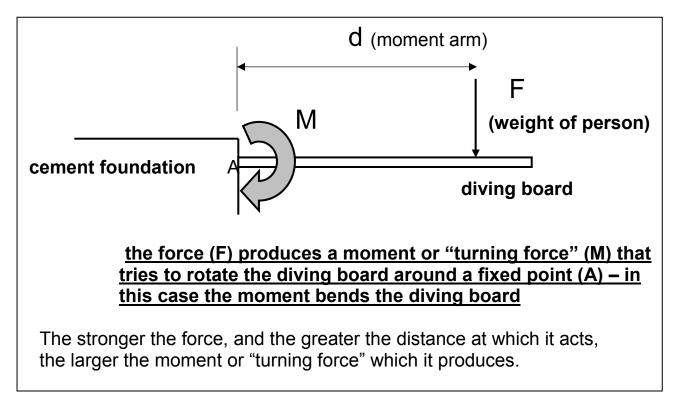
A moment or "turning force" (M) is calculated by multiplying a force (F) by its <u>moment arm</u> (d) – the moment arm is the distance at which the force is applied, taken from the fixed point:
