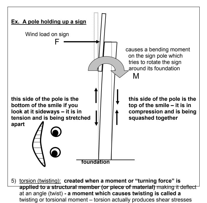
inside the material - a beam in torsion will fail in shear (the twisting action causes the molecules to be slid apart sideways)
