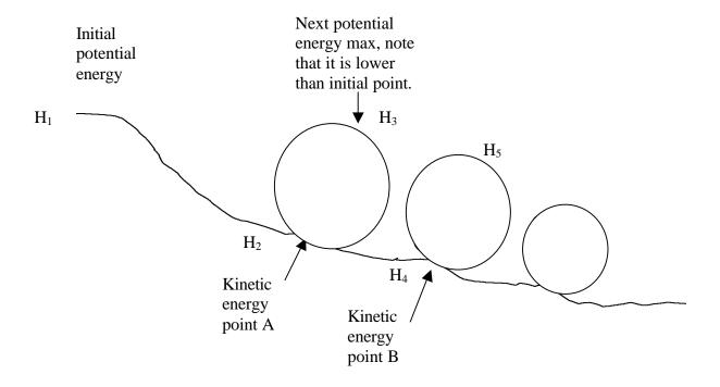
Ideal Kinetic Energy at point A  $KE = PE = (mass) x (H_1 - H_2) x (gravity)$
