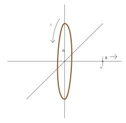
2. An extremely long straight wire carries a current of 15 A, and there is a circular loop of radius 3 cm along the wire as shown below. Approximating the wire as infinitely long, determine the magnitude and direction of the magnetic field at the center of the loop generated by the current.
