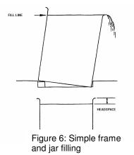
The simplest method is to fill containers from a jug that is calibrated for the correct volume. A funnel can be used to assist filling narrow necked bottles. A simple frame to tilt jars so that the correct filling level is achieved is shown in Fig. 6. At higher production rates a piston filler gives a uniform fill-volume and can be adjusted to fill different containers from 25-800 ml. This will also speed up the filling operation. taps into a 50 litre stainless steel bucket (Figure 7).
