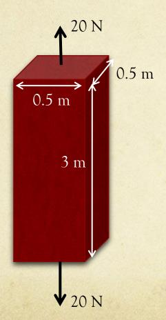
The rod below is exposed to a tensile force of 20 N and elongates by 0.03 m. Calculate the strain.
