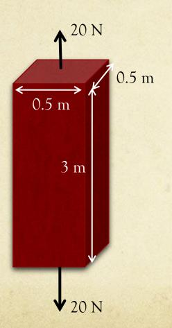
O This rod is exposed to a tensile force of 20 N. What is the stress in the rod?
