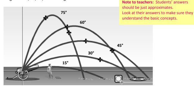
2. The image below shows the trajectory of a t-shirt launched from the cannon at 45 degrees and experienced *no* air resistance. Draw the trajectories of a t-shirt with air resistance if: a) it is rolled up into a ball first and stays that way, and b) if it is not rolled into a ball.
