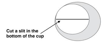
2. Using a straight edge, draw a line on the cup that is perpendicular to the slit, as shown below.
