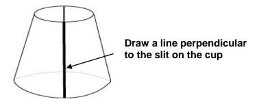
3. Place your diffraction grating into the slit on the bottom of the cup to complete your grating stand, as shown below.
