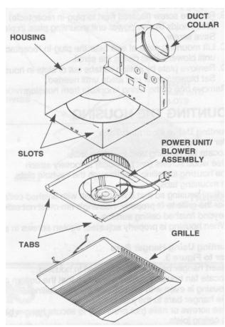
↑ Exploded view drawing of bathroom exhaust fan
