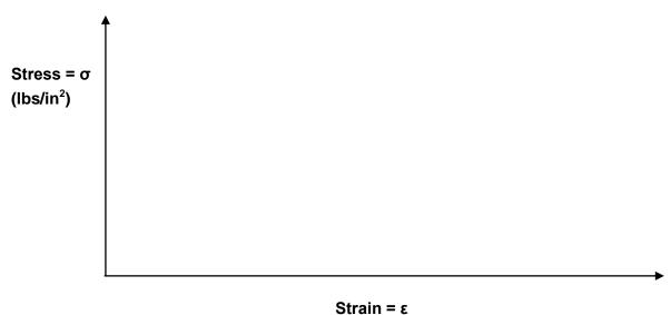
Modulus of elasticity (E) = rise ÷ run = Change in height between two data points ÷
